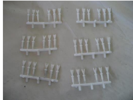
Figure 6. 3D printed moulds for manufacture of technical bellows (a) carbon fibre reinforced PEEK moulds (b) Pure PEEK moulds with moulded parts in position. (Images courtesy LIM Technics)
