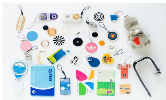
Figure 5: Different shapes and sizes of RFID tags
